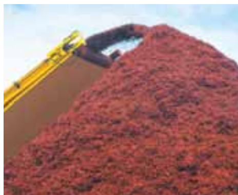
The ColorMaster® CM101 coloring system converts ordinary wood waste into profitable, color-enhanced landscaping mulch. The CM101 attaches to the fender of the trailed HG6000. A pump, two spray bars, and up to 19 colorant nozzles, powered by the grinder's hydraulic system, fuse liquid colorant into the wood fiber providing optimum coloring.
