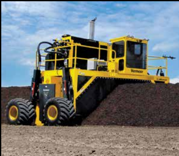
Both elevating-face and drum-style configurations define the Wildcat by Vermeer line-up of compost-turning equipment.
