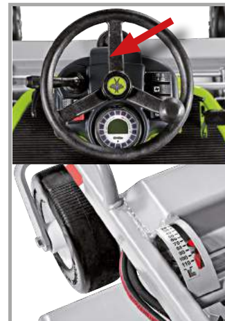
hydraulic assisted and continuous cutting adjustment
