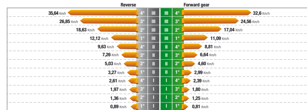
Graph of speeds in km/h of the AR and RS version tractor The graph highlights the progression of the gear ratios without any overlap of speed in any forwarding range.
