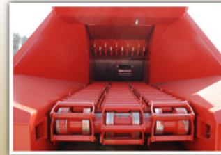
Infeed System Aggressive live floor and large top feedwheel with internal drive ensure positive feed of brushy tops and limbs.
