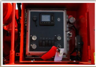
Morbark Integrated Control System The ultimate diagnostic system; monitors hydraulic pressures, temperatures, clutch systems and engine efficiency while automatically adjusting to maximize performance.
