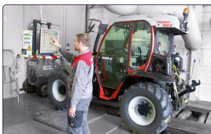
Before delivery, all vehicles undergo intensive functional testing such as here on the roller test bed (pictured).
