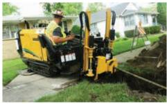
NARROW FOOTPRINT. This drill is 8.5" (21.6 cm) narrower in width than the next sized drill in the lineup and can get through a 36" (91.4 cm) gate or fit on a narrow trailer with other iobsite essentials.
