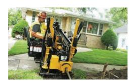
MORE POWER. Equipped with a 48 hp (35.8 kW) Kohler engine, this drill offers 1200 ft-lb (1627 Nm) of spindle torque and 7850 lb (3563.9 kg) of thrust/pullback.
