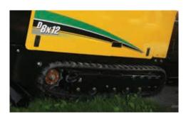
**TRACKS.** Tracks offer ideal traction for operation while providing minimal ground disturbance. This track system design allows a forward ground drive speed of 2.8 mph (4.5 km/h), which is 45% faster than the leading competitor.
