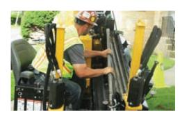
MULTIPLE ROD OPTIONS. Equip your drill with either a 6' (1.8 m) 1.66" or 1.31" (4.2 cm or 3.3 cm) Firestick® drill rod and save time on the job with 180' (54.9 m) of on-machine rod carrying capacity.
