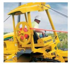
**Swiveling operator station**Hydraulic controls rotate with the operator seat to enhance ease of operation and visibility of the rear attachment.
