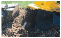
**CUTTER WHEEL.** High cutter wheel moves away from the machine as the boom drops, increasing the maximum cutting width. The SC852 gives you a cutting height of 31" (78.7 cm) above ground and 25" (63.5 cm) below — the deepest cut in its class.
