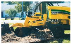
**CHIP CONTAINMENT.** Ground clearance allows plenty of room for chip containment, while the rounded chip blade moves chips around the jobsite easily, reducing the need for manual chip moving. A wide wheel base provides stability; a differential lock on the 4WD system can be disengaged for tight turning.
