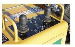
**OPERATOR PRESENCE SYSTEM.** The dual-axis joystick control handles for boom swing, boom raise/lower and machine propel are equipped with an operator presence feature. This user-friendly operator presence system is intended to enhance operator safety.
