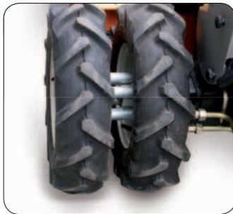
**Dual rubber wheels 5.0-10** for optimum performance on slopes (option)
