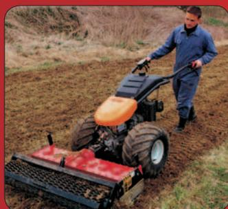
**Rotary harrow UK 75 / 90 / 100 / 125** with vertically adjustable grid roller, working width 75, 90, 100 and 125 cm
