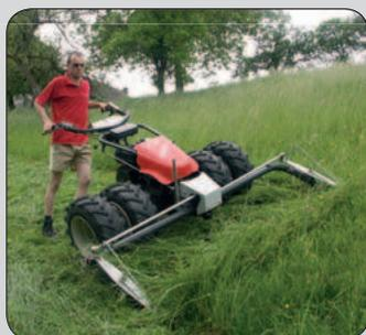
Even in extreme situations the non clogging **high clearance double knife mower** provides excellent mowing performance.
