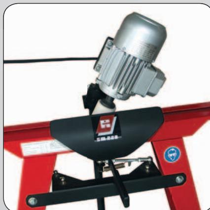
**Double-knife cutter drive with blade protection**
