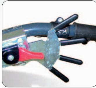
Mechanical travelling drive adjustment by means of a **smooth hand lever** (finger rake).
