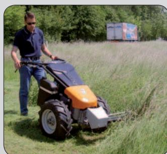
The **twin blade mower with lateral drive** is especially suited for mowing along embankments and guard rails.
