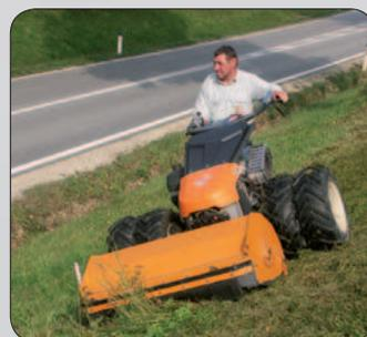
**The FMF 100 R flail mower** with rear roller and 6 mm blades is just the right appliance for professional applications.
