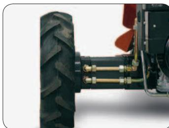
The **wide gauge assembly** is 280 mm wider and is excellent for slopes and cross country applications (only for M14).
