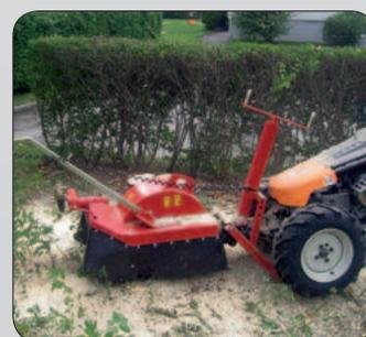
M14 with **SF 50 tree stump grinding cutter**, a powerful but manageable piece of equipment that you can continue to use even in tight spaces.
