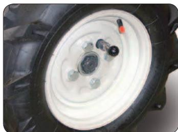
The **wheel cut off** is necessary for towing and makes it easier to manoeuvre the mower when the engine is switched off.
