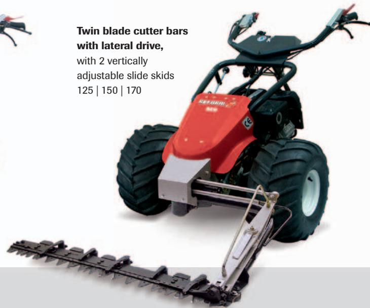
**Twin blade cutter bars with lateral drive, with 2 vertically adjustable slide skids**
