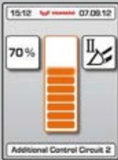
Electrical proportional adjustment of the hydraulic performance of the 3rd circuit.
