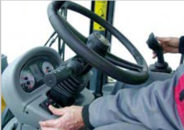
Electrical proportional adjustment of the hydraulic performance of the 3rd circuit.
