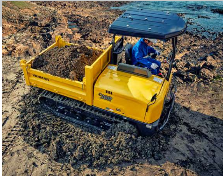
Spin turn by reverse turning both crawlers
