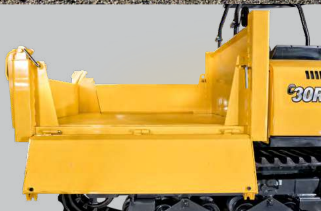
Three-side flaps wagon with rear dumping
