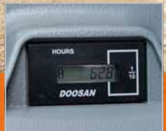
Hour meter (from ground level)
