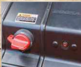
Battery cut-off switch
